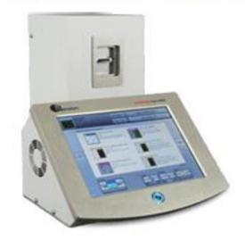
Cellometer Auto 2000 Primary Cell Viability Counter One-touch assays for analysis of a wide range of primary samples
