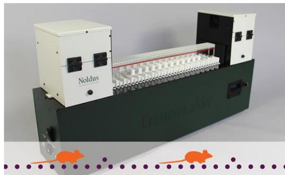
The ErasmusLadder is an automated system for testing laboratory mice for cerebellar deficits. It accurately measures and analyzes motor behaviors at different time points, allowing you to separate control and affected mice on basis of motor learning and motor performance abilities. It can also induce a cerebellar reflex during the test to specifically challenge that part of the brain.
